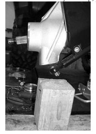
9) Lower the jack, this will place weight on the end of the strut that is connected to the control arm. This will compress the spring and strut. Fasten the two bolts on the back of the strut.
