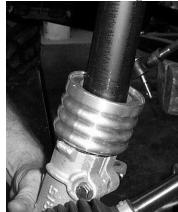
7) Once you have assembled the lift bracket in place and have loosely attached the strut to the strut cartridge. Insert the axle into the strut and attach the control arm to the bottom of the strut assembly.
