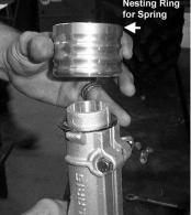
6) Slide the strut cartridge back into the socket.
