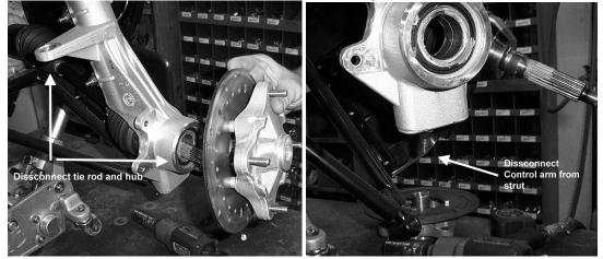
4) Leaving the top of the strut connected to the frame loosen the two bolts on the back of the strut. This will allow the strut to slide off the strut cartridge and away from the spring.
