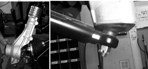
8) With the ATV still jacked up, place a block of wood or another solid object under the control arm.
