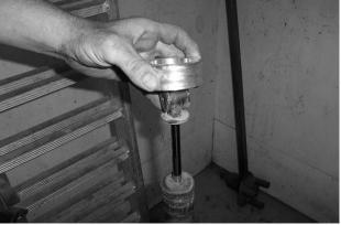
6) Place the spring back on the shock and compress it to reinstall the retaining clip.
