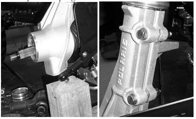
10) Reconnect the tie rod, hub, and brake assembly. Reconnect the hub assembly using the new castle nut provided in the kit. Leave off the factory conical washer. **Make sure to secure it with cotter pin.**
